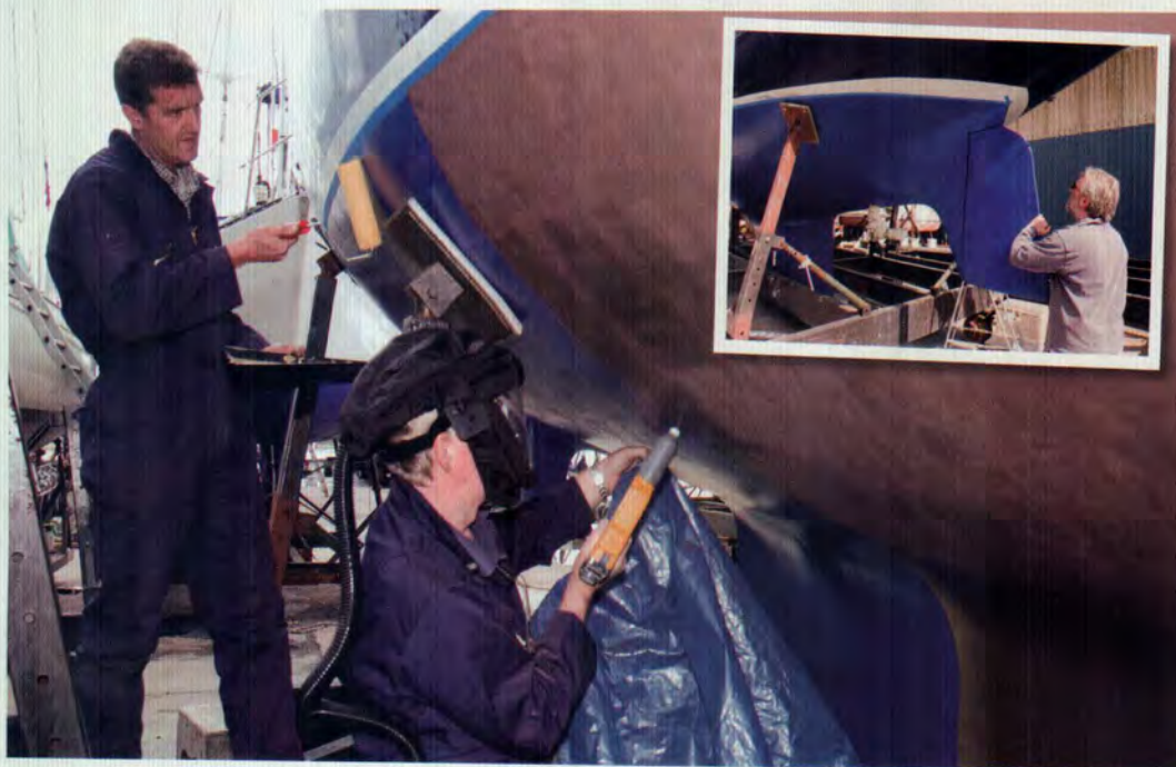
Long life, copper-rich systems, which apparently last for several years, have obvious attractions. The only obvious drawback is the fact that you need to get right back to the gel coat. It's also a job best left to the professionals.
