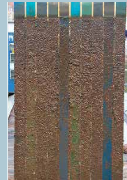
A board from Whitby as removed, showing how the slime ran off the two Seajet products, 038 and 033
